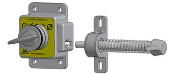
1. While the key is free, the bolt of the AI is trapped in the mechanism. The door is locked.
