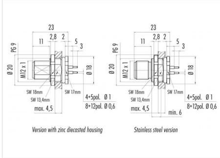
**Contact arrangement (Plug-in side)**
