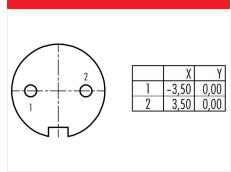
Contact arrangement (Plug-in side)
