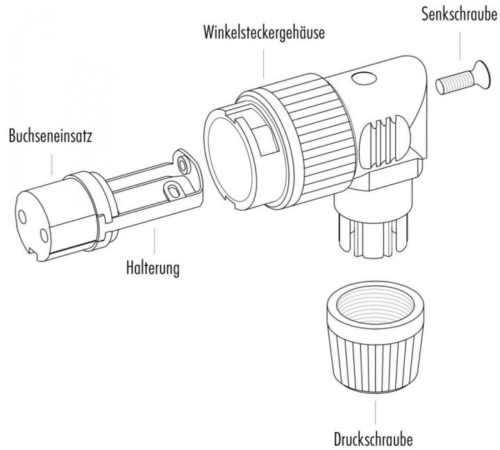
Product description **Bayonet female angled connector, Contacts: 16, 4.0 - 6.0 mm, shielding is not possible, solder, IP40**
