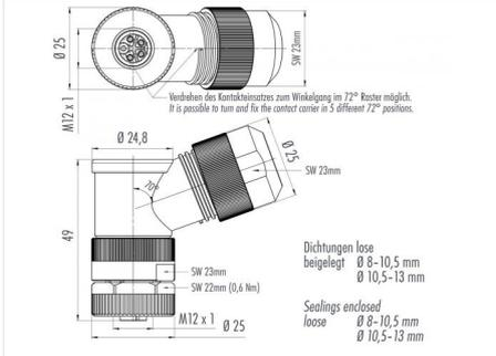
**Contact arrangement (Plug-in side)**
